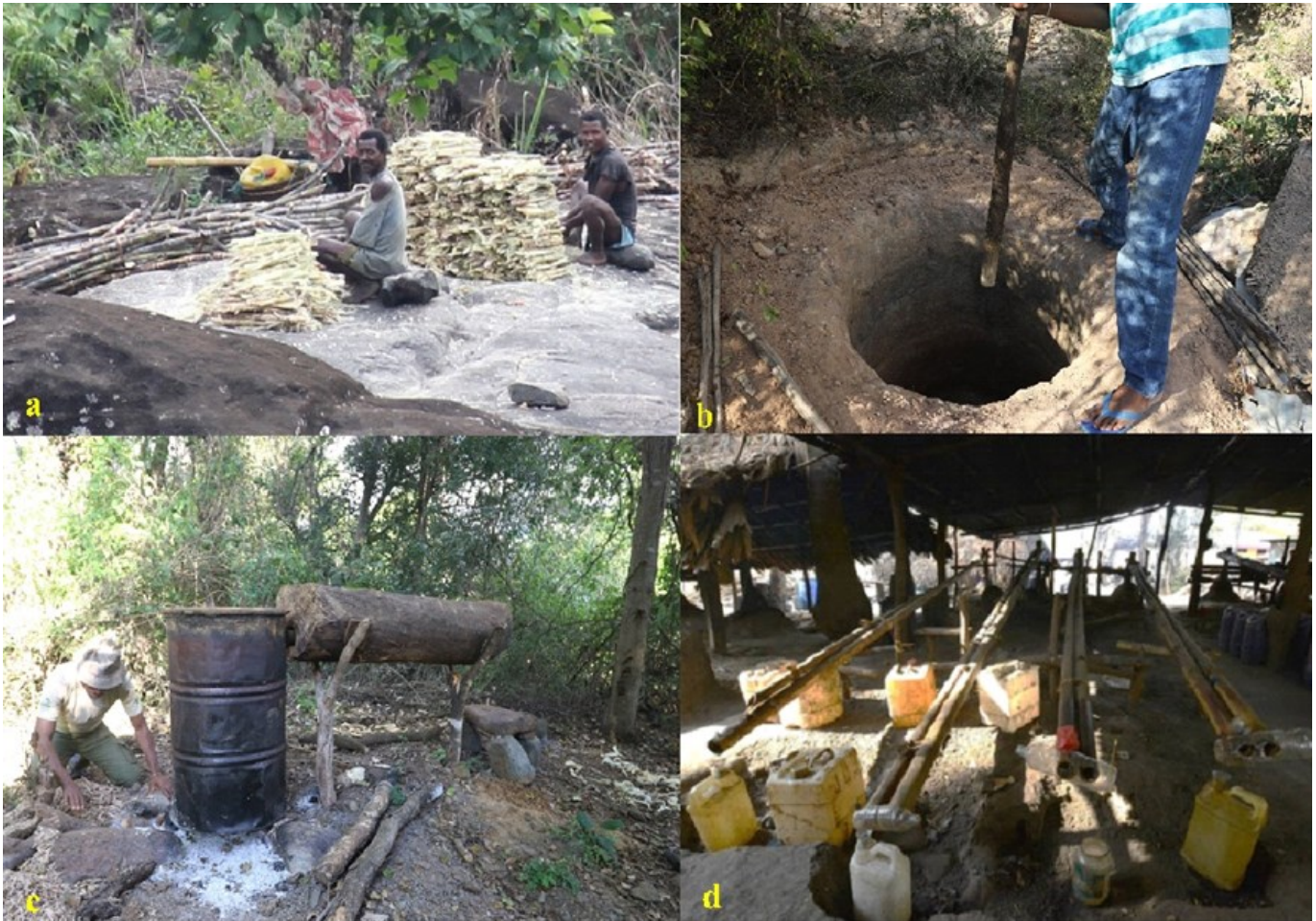
Figure 1 Production process of toaka gasy a) Collection and preparation of sugar cane b) Fermentation process with additives, c) Cooking and distillation with traditional alembic, d) Recuperation of toaka gasy (photos by authors).
